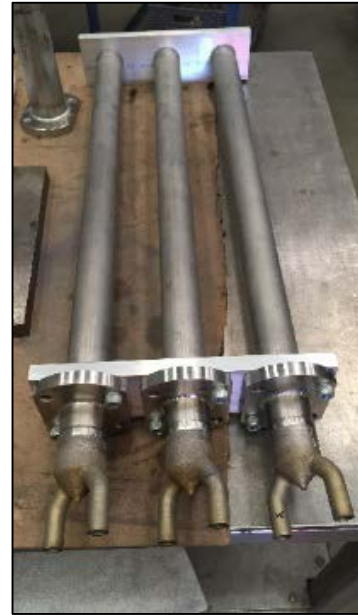
SCO 2 manifolds and in-bed heat exchanger assembly
